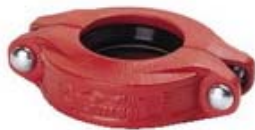
1NR-Reducing Coupling 65x50 - 200x150mm 2 ½"x2" - 8"x6"
